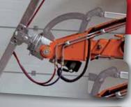
The lifting head has two settings, adjusted by means of two holes for the locking bolt. The lifting head can therefore be adjusted to tilt more towards the ceiling or floor.
